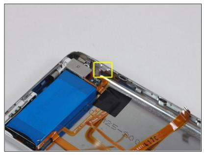
Now to repair the damage caused by liberating the internal parts of the iPod Classic! It is highly likely that at least one of the metal clips in the rear panel has been bent upward. These clips must all be pointing downward in order to reinstall the rear panel.
