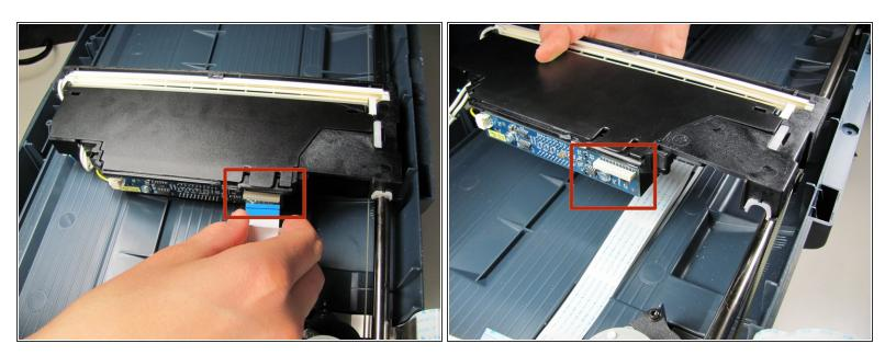
Detach the white ribbon wire from the scanner head by pulling gently at the connection.
