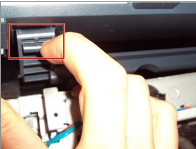
Press down on the two plastic hinges to remove the upper portion of printer.
