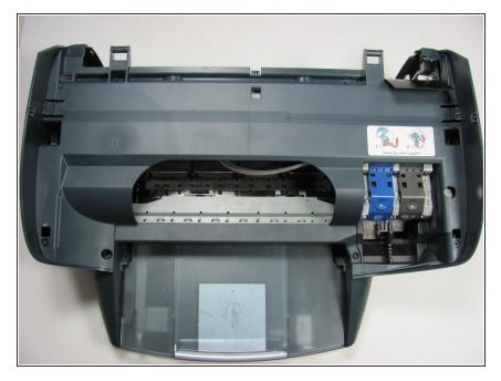
Detach the scanner tray from the printer by lifting the scanner tray off the printer body.
