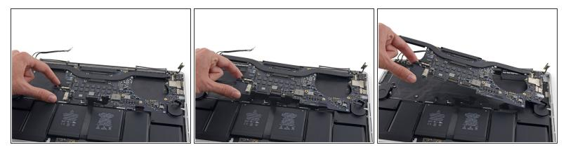
• Lift and pull the entire logic board assembly away from the wall of the upper case.
