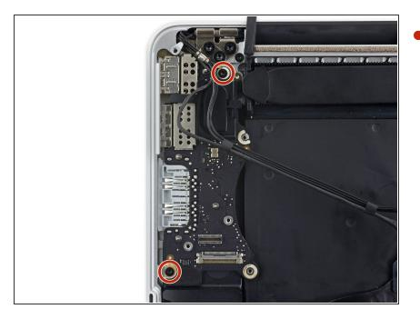
Remove the two 3.1 mm T5 Torx screws from the I/O board.
