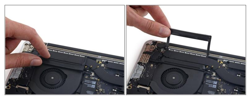
• Peel the right rubber cover up off the fan and fold it out of the way.
