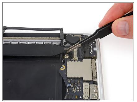
• Remove a small rubber cap off the screw at the end of the heat sink.
