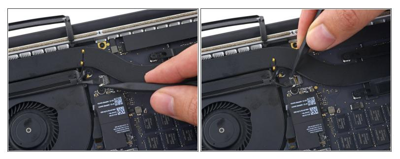
Use the tip of a spudger to push the camera cable connector out of its socket on the logic board.
