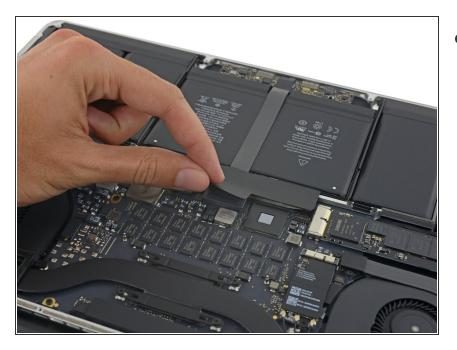
Peel back the sticker covering the battery connector.
