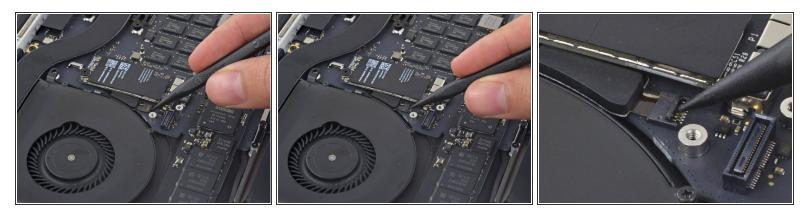
• Use the tip of a spudger to flip up the retaining flap on the right fan ribbon cable ZIF socket.
