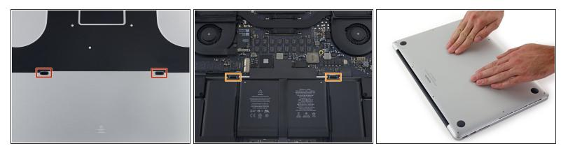
(i) The lower case has two plastic pegs (red) that fit into plastic clips in the upper case (orange).
