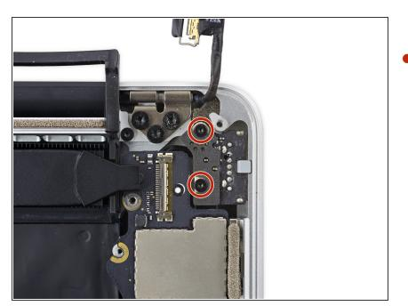
Remove the two 4.0 mm T5 Torx screws from the MagSafe 2 board.
