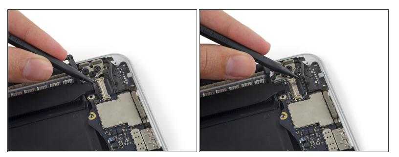
Use the tip of a spudger to flip up the display data cable lock and rotate it toward the MagSafe 2 power port side of the computer.
