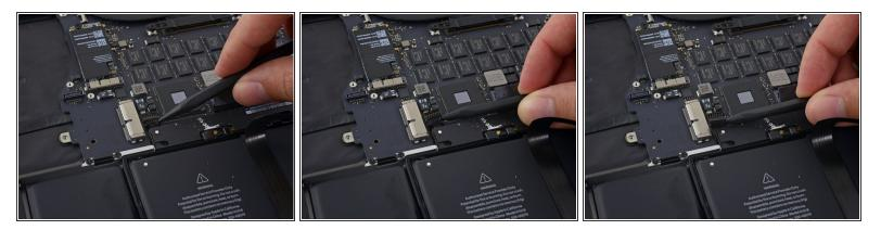
Use the tip of a spudger to pry the right speaker connector up and out of its socket on the logic board.
