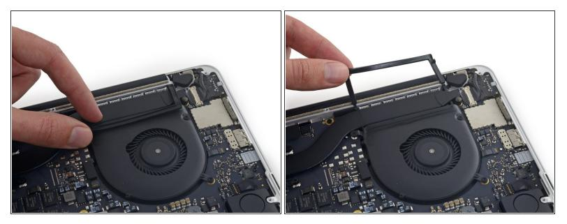
• Peel the left rubber cover up off the fan and fold it out of the way.
