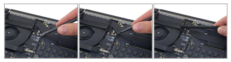
Use a spudger or tweezers to pry the three AirPort antenna cables straight up off of their sockets on the AirPort board, and bend them up and out of the way.
