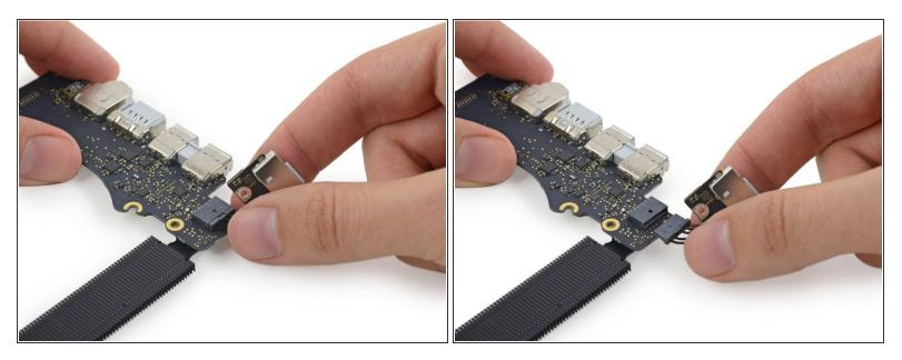
• Pull the MagSafe 2 connector straight out of its socket (parallel to the logic board).
