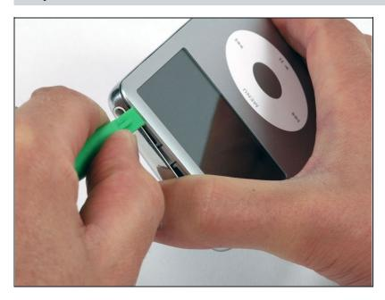
Near the other top corner, insert an opening tool into the seam between the front and back of the iPod
