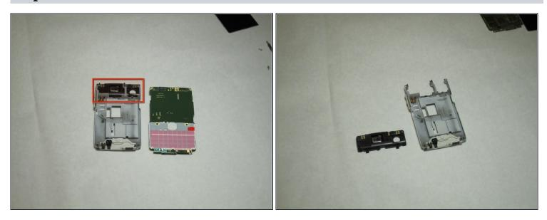
• After the logic board has been removed, there is nothing else securing the antenna to the back cover. Simply remove the antenna by pushing outward from the interior side.
