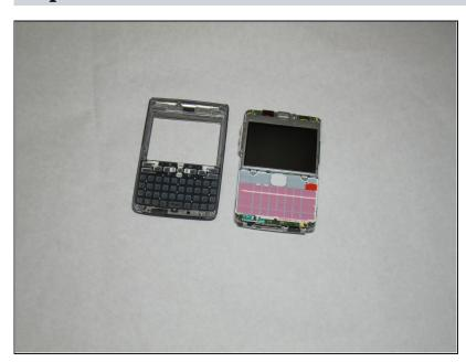
• Remove the cover by pulling it up and off.
