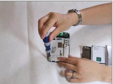
• Remove the four screws that secure the front cover to the rest of the phone using a T7 screwdriver.
