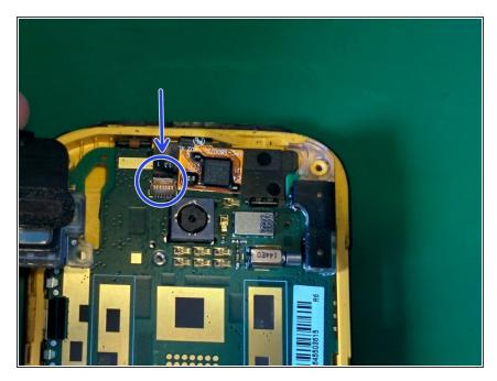
Disconnect the digitizer cable from is socket, flip the brown clasp up from indicated edge and gently remove the cable.
