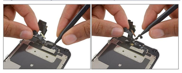
• Holding the front-facing camera out of the way, use the point of a spudger to push the ambient-light sensor up out of its recess in the front panel.
