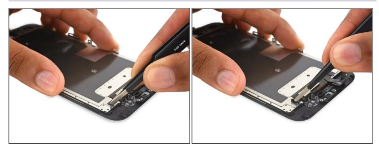
Use a pair of tweezers to peel up the piece of tape from the EMI shield, near the front camera housing.
