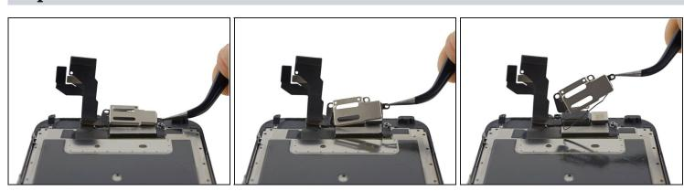
Lift up and remove the earpiece speaker bracket, peeling up the bracket gasket as you go.
