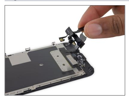
Remove the front-facing camera and sensor cable.
