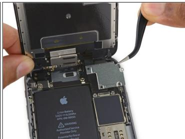
• Remove the display cable bracket.
