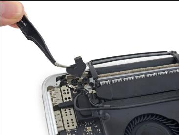
Remove the two rubber hinge covers.
