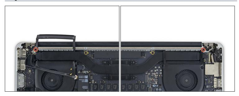
Remove the two 3.2 mm T5 Torx screws securing the aluminum hinge covers to the upper case.
