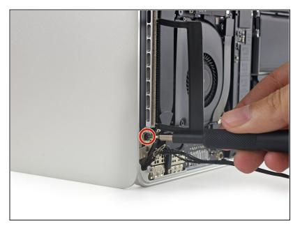
While holding the display and upper case together with your left hand, remove the remaining T8 Torx screw from the lower (closer to the table) display bracket.
