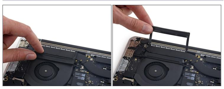
• Peel the right rubber cover up off the fan and fold it out of the way.
