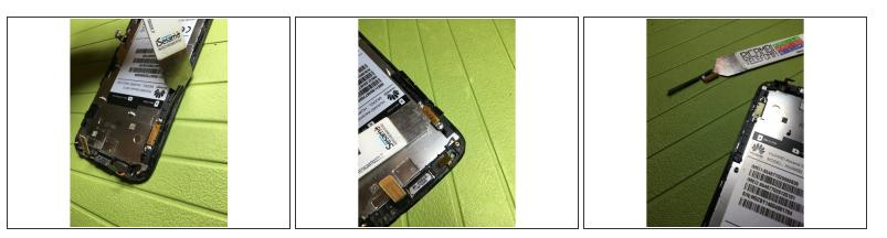
• Using the phone for leverage, remove the flat volume keys and turn off the device.
