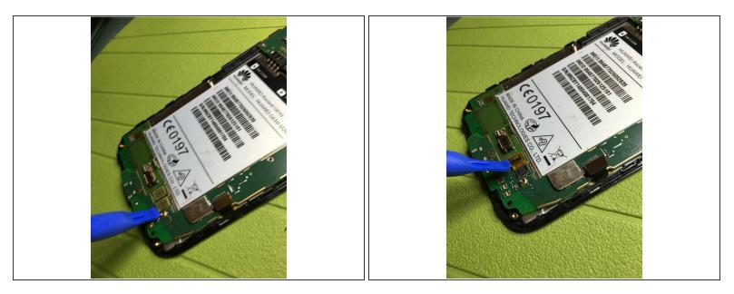
• Unplug the connector that joins the two boards.
