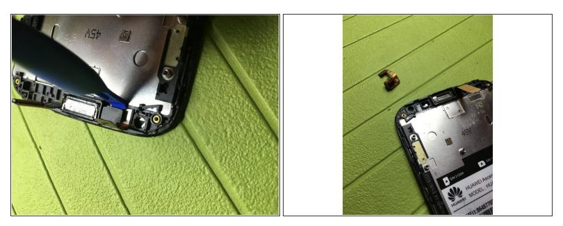
• Remove the ambient light sensor.
