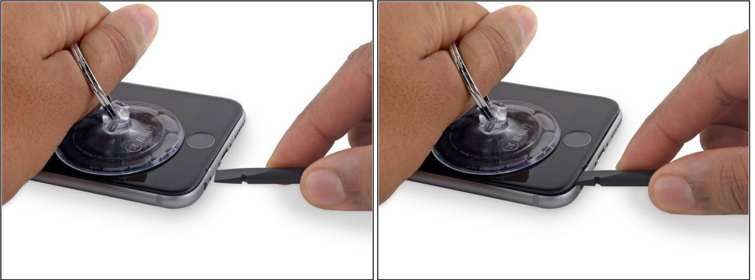
ⓘ There is a notch on the underside of the display, just above the headphone jack. This is the safest place to begin prying the phone open.
