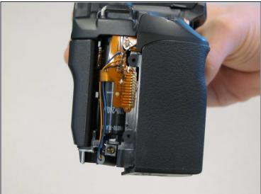
• Slide the panel toward the bottom of the camera to remove.
