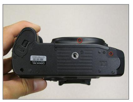
Remove the 4.3 mm black screw under the lens ring, and the 4.8 mm black screw under the camera.
