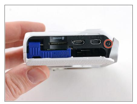
Use a Phillips #00 screwdriver to remove the 4 mm screw inside the battery compartment.
