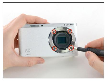
• Remove the four 5 mm Phillips #00 screws from the lens assembly.
