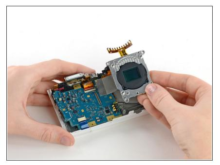
• Gently remove the sensor mount from the camera case.
