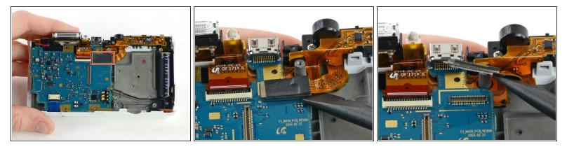
• Use a spudger to disconnect the LCD ribbon cable by prying it straight up from the motherboard.
