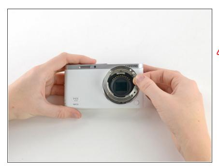
• Remove the metal lens mount by hand or with tweezers.
