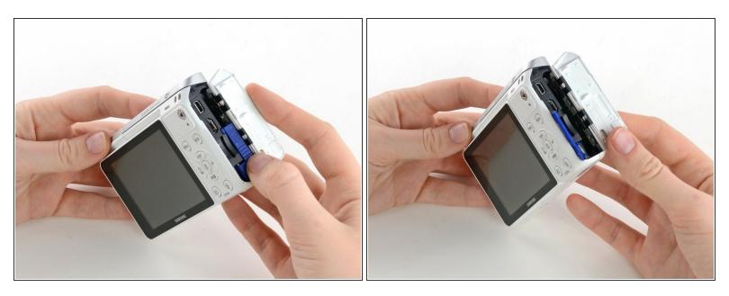
• Push the blue trapdoor to the left to release the battery, and remove the battery.
