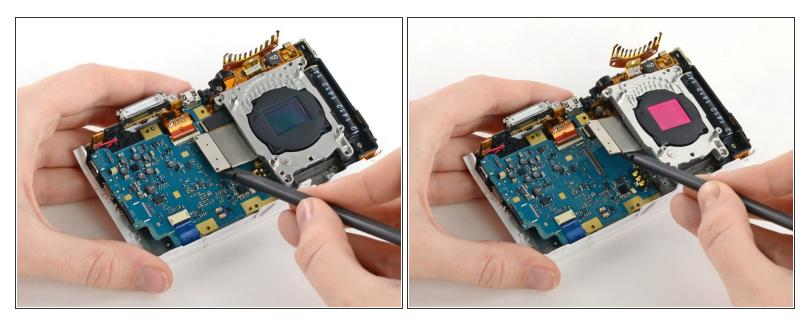
• Use a spudger to disconnect the ribbon cable connecting the image sensor to the motherboard.
