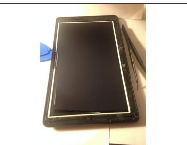
The part number on the LCD cable is TPV-AM070NB02A.
