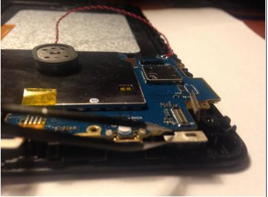
Use heat and tweezers to lift the Power Button cable from the plastic frame.
