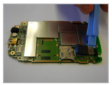
Remove the camera lens from the motherboard using the plastic opening tool.
