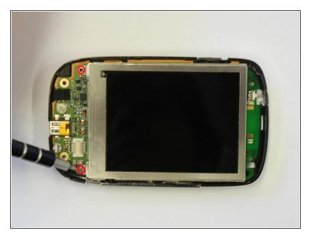
Unscrew the torx-head screws at the base of the LCD screen using the T5 Torx Screwdriver.
