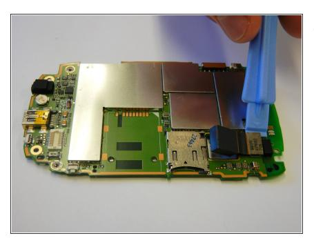
Remove the camera lens from the motherboard.
