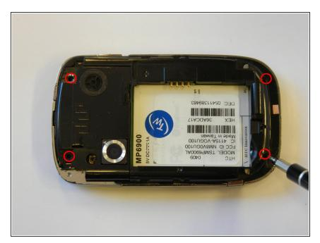
Remove the 4 torx-head screws in the corners of the phone using the T5 Torx Screwdriver.
