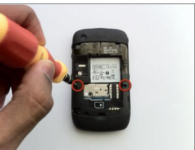
Remove the two Torx T6 screws to the left and right of the battery.
