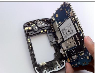
Using a plastic opening tool, gently pry the motherboard assembly from the device's frame.
