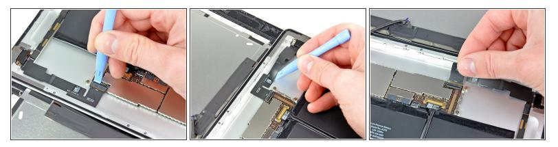
• Use the flat end of a plastic opening tool to flip up the retaining flap on the headphone jack and front-facing camera ribbon cable ZIF socket.
