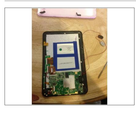
Next the following highlighted spots are screws. These screws must be loosened to separate the motherboard and digitizer from the outer glass components. Remember lefty loosely, righty tighty. All screws were placed on a magnet board to ensure they did not roll away
