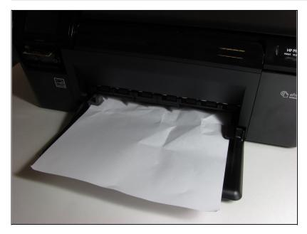
Identify the location where the piece of paper is jammed.
