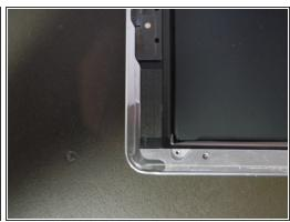
Pliertek wall mold attached; corner mold below.
