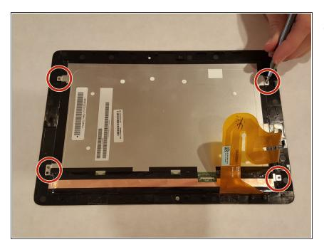
Remove the 4 screws around the metal portion of the screen (this is the LCD display).
