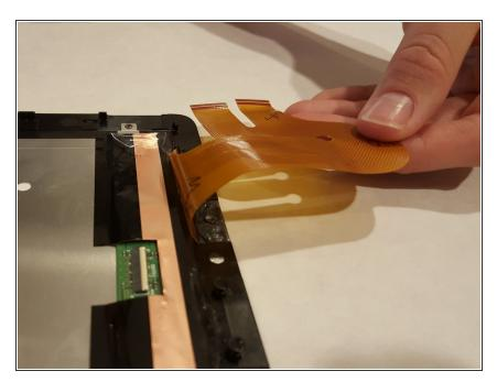
Peel the orange ribbon back (it has adhesive sticking itself to the black electric tape looking stuff surrounding the metal portion).
