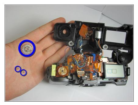
On the bottom side of the top bezel, remove the ring, detent ball and spring. Your control dial is now ready to be replaced with a working unit.
