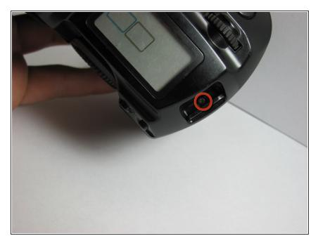
Remove the 4.3mm screw below the camera strap ring.
