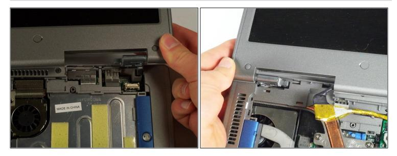
• Lift the display module directly upwards from the base of the computer.
