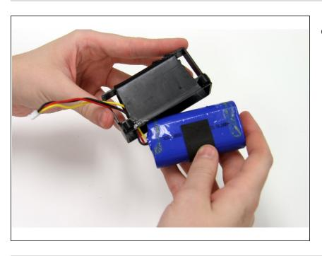
Slide the blue battery out from the black container. Your battery is now removed from the device and is ready for replacement.
