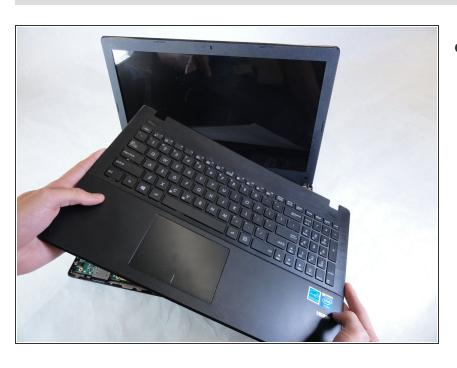
Remove the fully disconnected keyboard module from the laptop. To reassemble your device, follow these instructions in reverse order.
