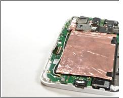
Remove LCD connector by lifting the black plastic flap.
