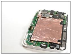
• Remove LCD connector by lifting the black plastic flap.
