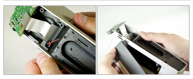
Carefully pull on the battery cover until the rubber tab slides out of the aluminum casing.
