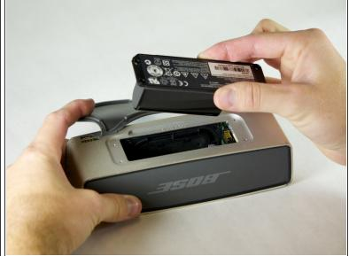
• While holding the cover back, pull straight up on the battery to remove it.
