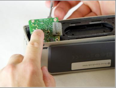
Remove the circuit board by pushing it with your index finger in the direction shown while using a nylon or metal spudger to lift it up and out of place.
