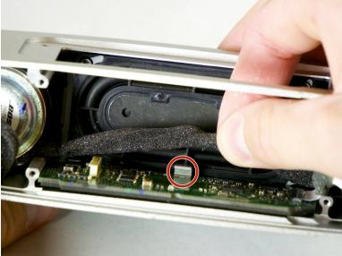
Unhook the speaker wires clipped onto the button switch circuit board.
