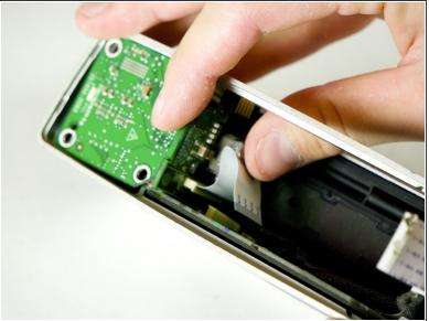
Reach through the battery compartment hole and unplug the power strip shown.
