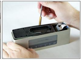
Use a Metal Spudger to pry up the plastic divider.
