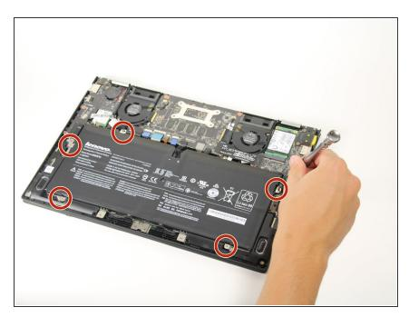
Using a Phillips #00 Screwdriver, remove the five 5/16" screws surrounding the battery.
