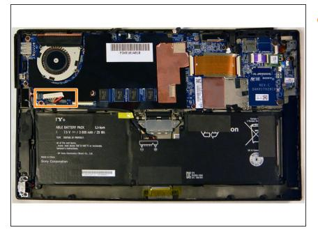
Disconnect the battery from the motherboard by pulling out the cable below the fan.
