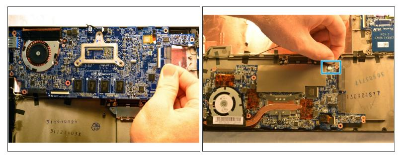
• Gently pull the motherboard out by pulling from the right side of the board and flip it so that the motherboard now sits where the battery was and the underside is now visible.
