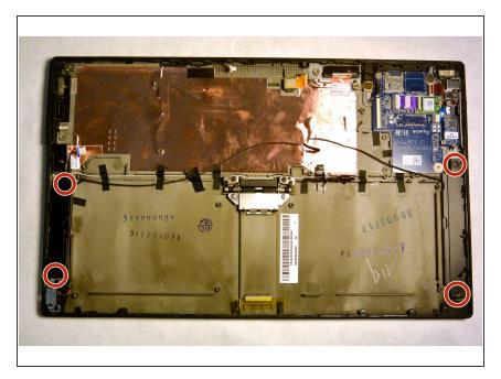
Remove the four 3 mm Phillips #000 screws from the upper and lower ends of each speaker module.
