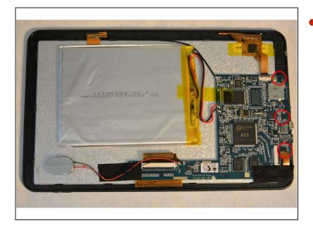
• Use the Phillips #00 screwdriver to remove the three screws from motherboard.
