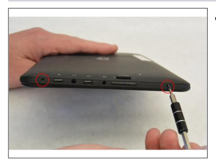
• Remove the two Phillips #00 screws from the bottom of the case.
