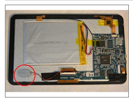
Pull the speaker away from the tablet. It should easily come off, as it is held on with a magnet.
