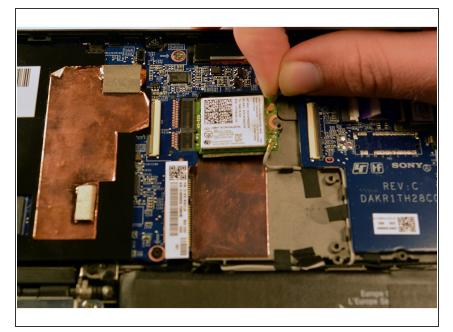
Remove the black and grey antenna cables from the right side of the device.
