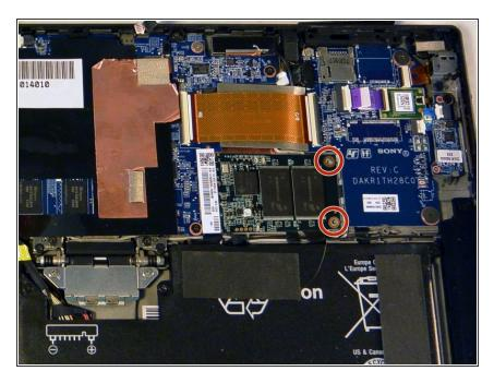
Remove the two 3 mm Phillips #000 screws from the right edge of the SSD.
