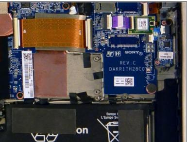
Pull the SSD towards the right and slightly up, removing it from the back assembly.
