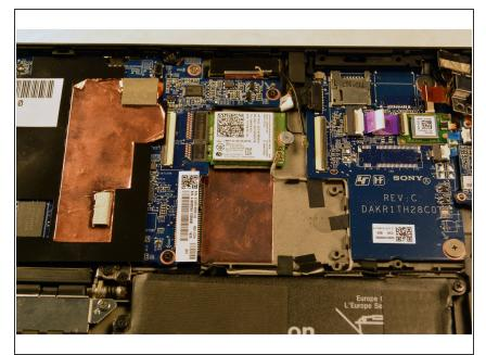
Remove the grey foam separator that was underneath the orange ribbon cable.
