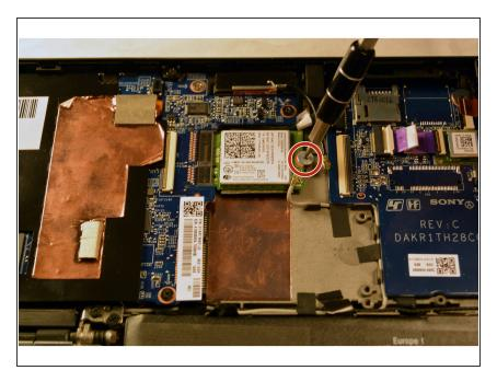
Remove the silver 3 mm Phillips screw that holds the WiFi module in place.
