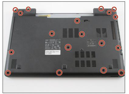
Remove all eighteen 8 mm screws with a Phillips #0 screwdriver.
