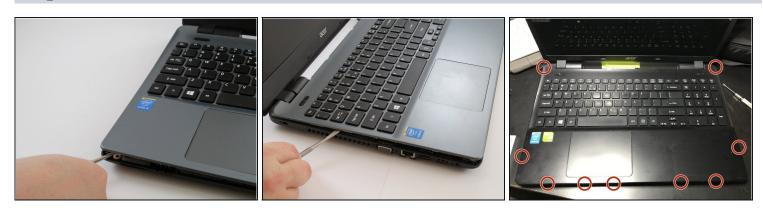
• Carefully pry apart the clips holding the keyboard in place by moving a metal spudger along the seam.
