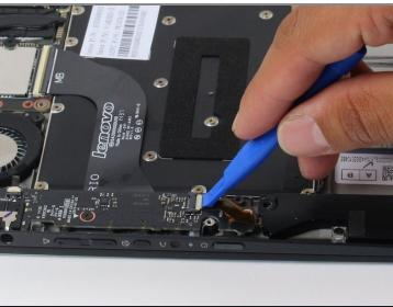
Using the plastic opening tool, flip open tab as shown.
