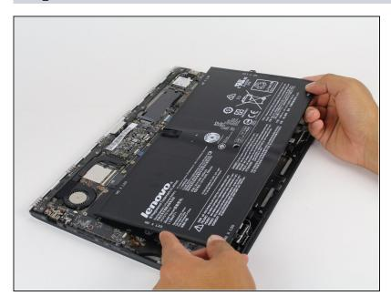
• Carefully lift and remove the battery.
