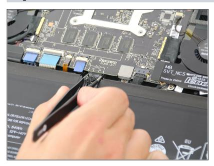
Using either tweezers or your fingers, disconnect the black battery cable by pinching either side of the connector and pulling towards the battery.
