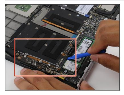
Remove the USB assembly using the plastic opening tool.
