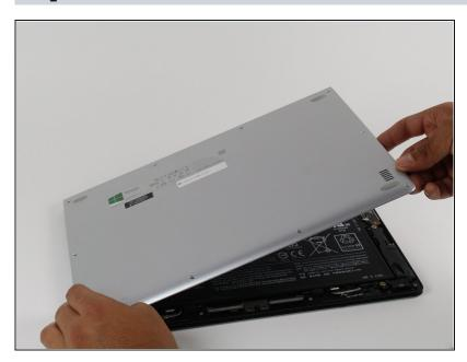
Remove the panel and place it in a safe location.
