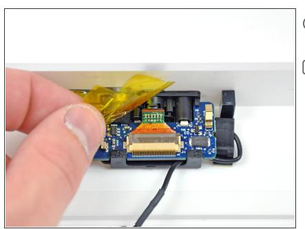
(i) If necessary, remove the strips of tape covering the camera board.
