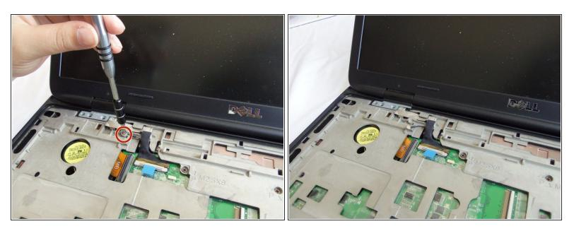
Loosen the grounding screw attached to the black monitor cable with a Phillips screwdriver.
