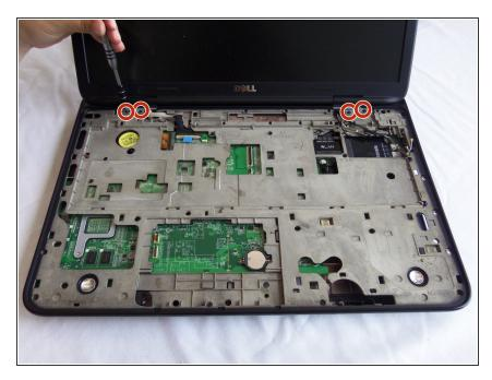
Unscrew four the 8mm screws directly under the keyboard with a Phillips screwdriver.
