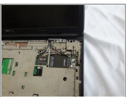
Gently remove the wires for the WLAN and WWAN cards from their housing.
