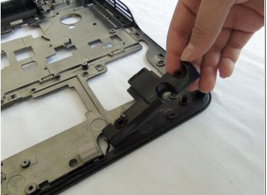
Gently lift and remove the right side speaker piece out of its casing.
