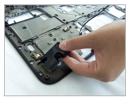
Gently lift and remove the left side speaker from its housing.
