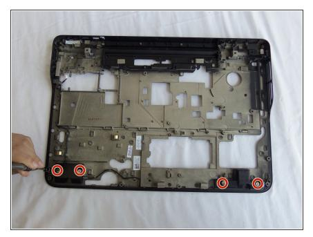
Unscrew four 4mm flathead screws with a Phillips screwdriver
