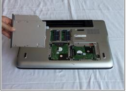
Using a plastic opening tool, pull out the optical drive.
