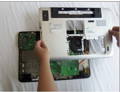
Holding the opening from the optical drive in one hand with the other hand holding the opposite side of the laptop, lift and remove the back cover assembly.
