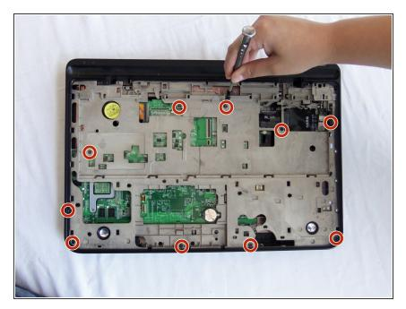
Unscrew the ten 8mm screws from the grey inner casing with a Phillips screwdriver.
