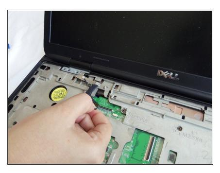
Gently remove the monitor cable from its holdings from the board.
