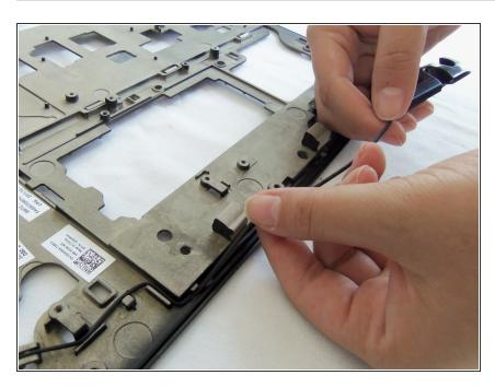
Carefully remove the wires from the holdings.
