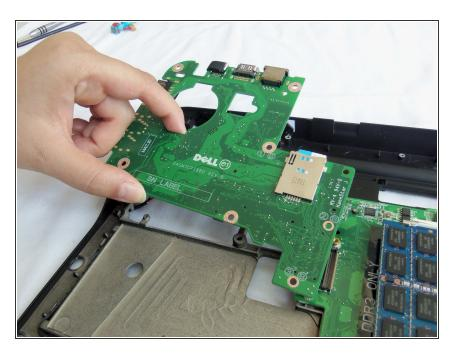
Lift and remove the Wi-Fi circuit board.
