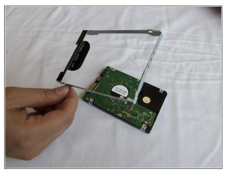
• Remove the hard drive casing.
