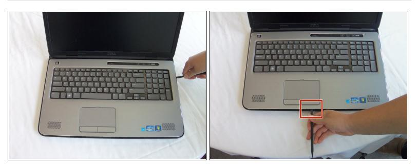
• Slide the spudger around the palm rest to release the clips.
