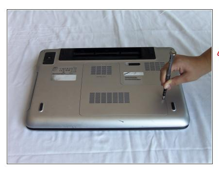
• Loosen the module cover screw with a Phillips screwdriver.
