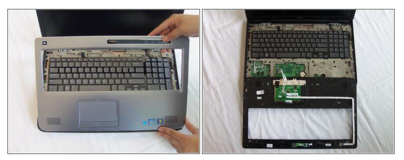
Gently lift and rotate the palm rest panel until it's upside down as it is still connected by the mouse pad wires.
