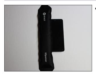
Lay the iOpener on side 1 of the phone for 90 seconds before attempting to open the front panel
