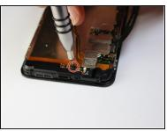
• Unscrew the four 2mm screws along the right side of the motherboard with a philips head
