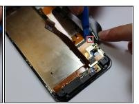
• Disconnect the 9 cables along the top and right side of motherboard using the plastic opening tool
