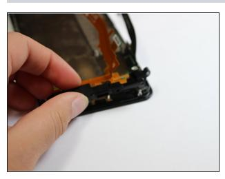
• Lift off bottom plastic piece with flat antenna cables
