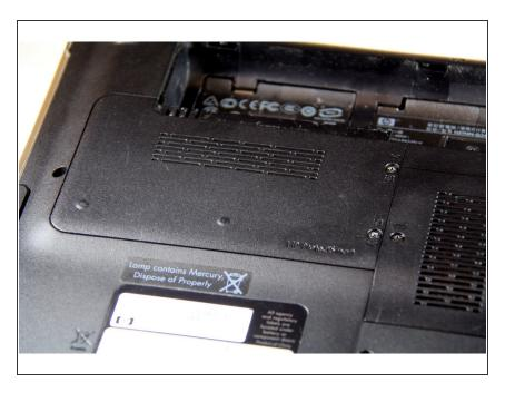
Identify the hard drive compartment, located at the top left-hand frame of the laptop.
