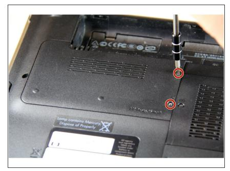
In order to remove the hard drive compartment cover, first remove the two screws located on the panel, using a size 0 Phillips head screwdriver.
