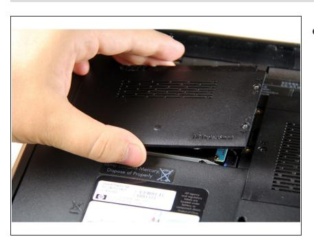
Expose the hard drive by lifting the drive cover.
