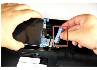
• Firmly hold both the black plug, and the hard drive itself to separate the drive from the cable.
