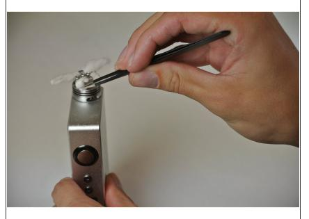
• Tuck cotton underneath coils and into the well of the atomizer using the tweezers.
