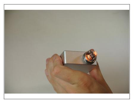
• Press the biggest button on vape to heat up coils until red hot.
