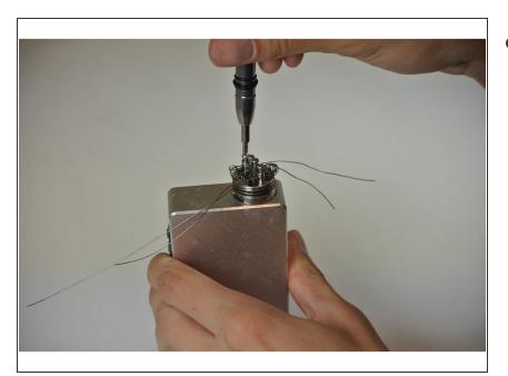
• Tighten the screws completely once coils are in desired position.
