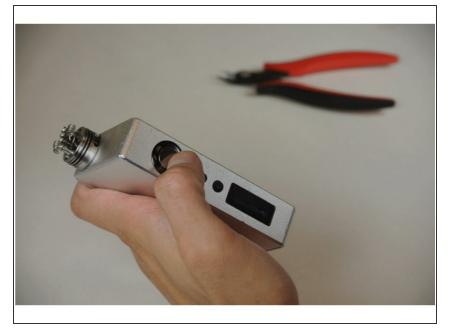
Re-insert the batteries and press the large button 5 times quickly to turn the vape on.
