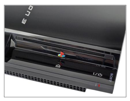
Now when the PS3 is in standby mode, hold the power button down until you hear it beep about 2 or 3 times, then release the power button.
