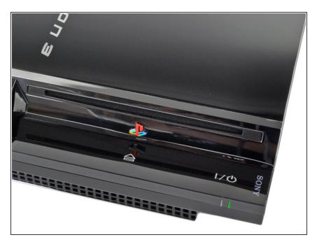
While the PS3 is on (green LED on), put the PS3 into standby mode (red power LED) by pressing the power button for 5 seconds.
