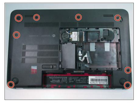
Remove all highlighted screws with PH 1 screwdriver. These screws are PM 2.0x2.5.
