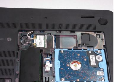
Very carefully, remove the SSD by gently pulling away from the SSD socket.
