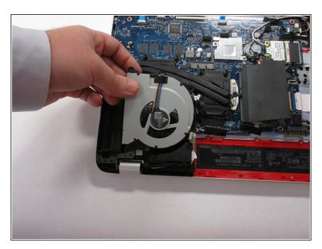
Remove the fan by sliding it out and pulling it upwards. Set the fan off to the side to reveal the connector.
