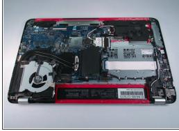
Pry open back plate area with plastic opening tool. The back plate should pry open with relative ease. If you feel some resistance at any point please refer to steps 2-5 because a screw has probably been missed.
