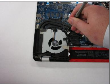
■ There are 3 screws holding the fan in place. These are PM 2.5x4.5 screws
