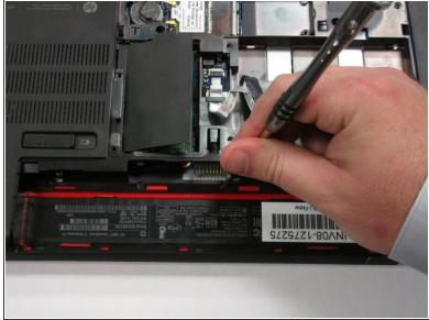
Remove all highlighted screws from the battery access area. These are PM 1.5x2.0 screws
