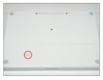
• Use a coin or spudger to rotate the battery-locking screw 90 degrees clockwise.
