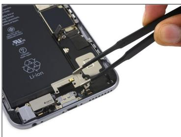
• Remove the Taptic Engine cable bracket.
