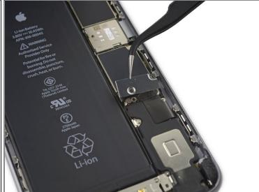
• Remove the battery connector bracket.
