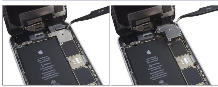
• Remove the display cable bracket.
