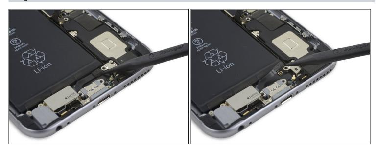
• Disconnect the Taptic Engine's flex cable from the socket on the Lightning Connector flex cable.
