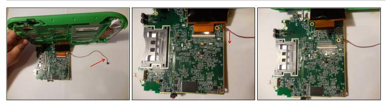
• Lift the motherboard up exposing the fourth and final wire. Once you lift up the motherboard you will need to pull down on the wire to disconnect.
