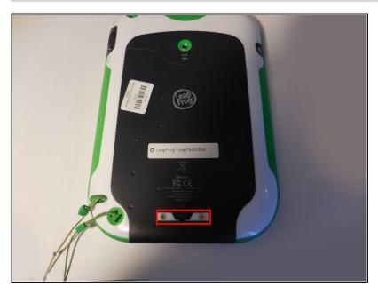
Remove the barcode covering the two screws on the lower back of the Leap Pad.
