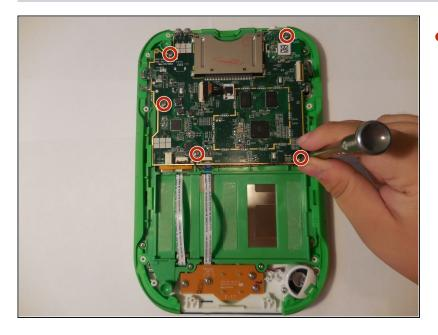
• Unscrew the five screws holding the motherboard into the housing.
