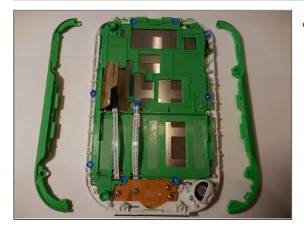
• Using the screwdriver with the PH1 bit, unscrew all nine of the exposed screws holding the plastic base down and remove the base.
