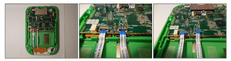
• Disconnect the three wires that will be visible on top of the motherboard. The wires need to be disconnected by pulling them up vertically.
