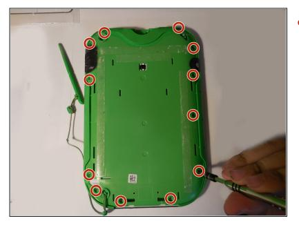
Remove the 7 mm screw to the right of the cartridge dock, two 8 mm screws in the top left, and the nine 8 mm screws holding the the green shell.
