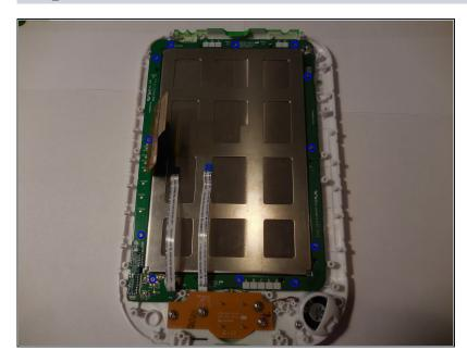
• Using the screwdriver with the PH00 bit, unscrew the twelve screws holding the screen casing down.
