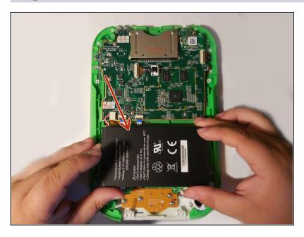
• Remove the hard plastic casing, exposing the motherboard and battery.
