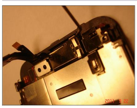
Use an automotive pick tool to lift the bracket up on the side of where the speaker lies. Slight upward pressure, do not force or pry.
