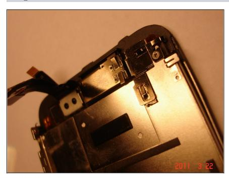
Lift the digitizer and LCD connectors and snap in the bracket/ribbon combo to finish it off.
