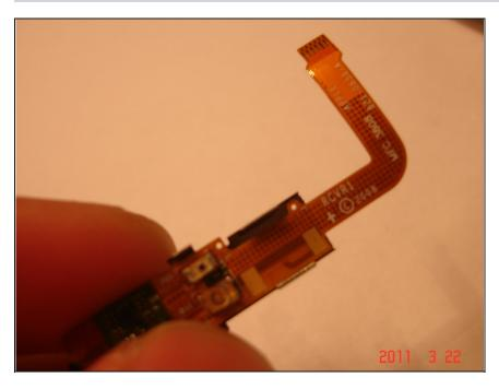
Peel off the adhesive backing protectors from the new ribbon, and line up the holes in the ribbon with the ones on the bracket as so.
