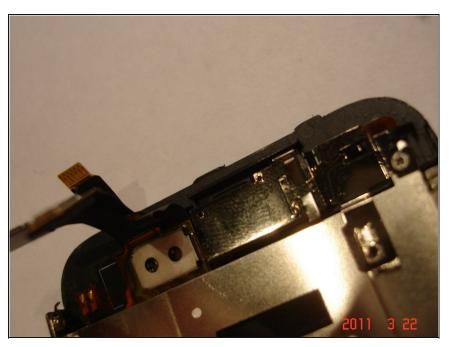
Remove the screw that holds this bracket in and put it in a safe place.
