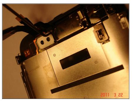
• Do the same with the other side and on the bottom of the bracket. This is held in with tension on fingers that clip into the screen midframe.
