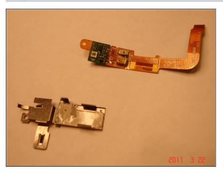
Peel the old ribbon from the bracket, note the orientation.
