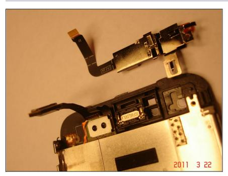
Once the bracket is loose, you can pull it up carefully maneuvering it up and around the LCD and digitizer connectors.
