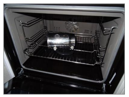
• Heat up to 50°C/120°F in oven in order to make the clips inside smooth.
