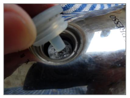
• Carefully embed the thermal contact in conducting paste. Then press bottom into body until you hear a clic three times. At last switch must be pressed in.
