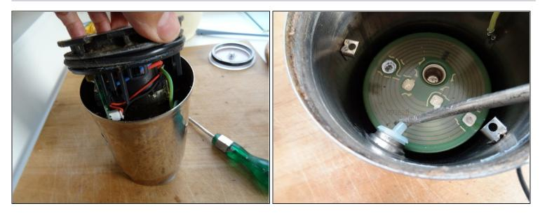
• Pull out the circuit board and the motor. After module is removed the on/off pad must be pressed in/through
