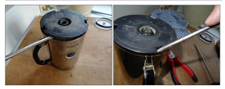
• Open the bottom with a strong screwdriver. Be careful not to break the clips inside
