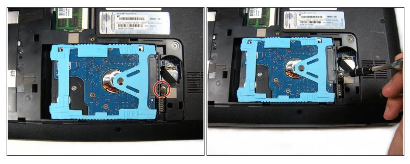
Use the PH 00 screwdriver to unscrew the 2.5 mm screw to the right of the hard drive.
