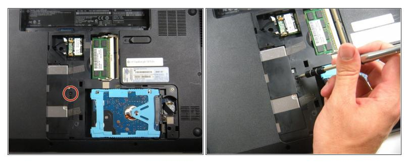
• Using the PH 00 screwdriver, remove the screw left of the CD drive.
