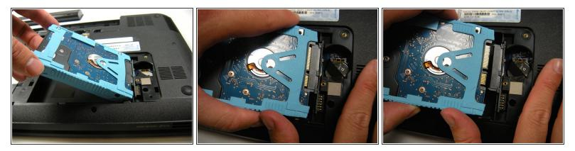
Pull the triangular blue tab to diconnect and remove the hard drive. You can see the word 'Pull' on the cover.
